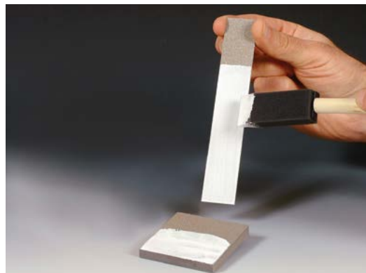
Ceramacoat™ 503-VFG-C-WHT applied to thermal spray substrate.
