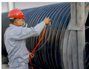
HiE-Coat™ 840-M coats industrial heat exchanger.
