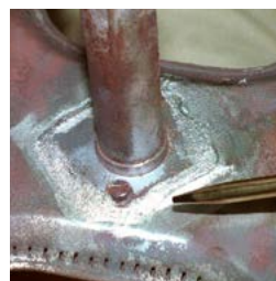
Pyro-Putty® 653 seals corroded burner manifold.
