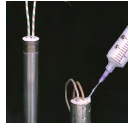
Ceramacast™ 586 pots ignitor and cartridge heater.
