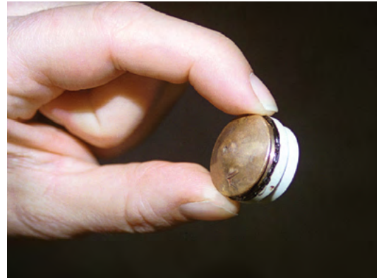
Aremco-Bond™ 570 bonds ceramic to copper nozzle.
