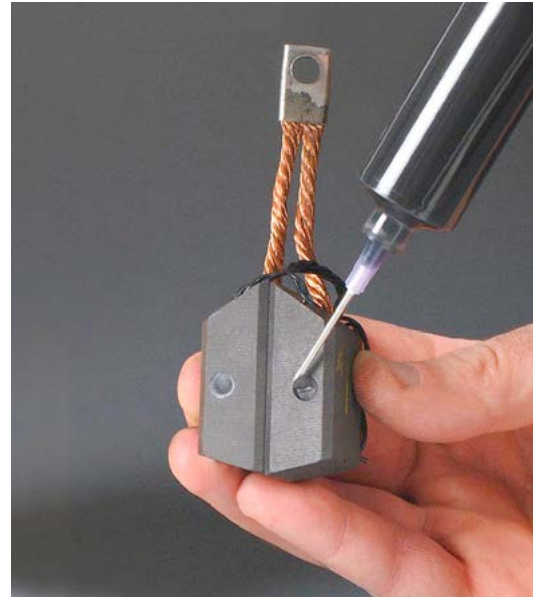
Graphi-Bond™ 551-RN seals sensor in carbon brushes.
