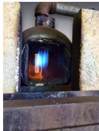
HiE-Coat™ 840-CX applied to a gas-fired forge.
