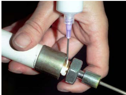
Ceramabond™ 671 used as a high temp threadlocker.
