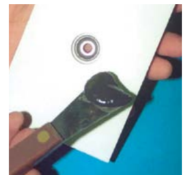
Aremco-Bond™ 2150 bonds ceramic wear tile.
