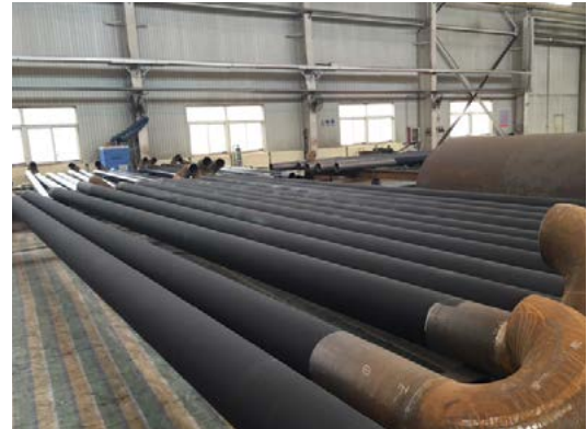
HiE-Coat™ 840-M coats gas-fired heating tubes.
