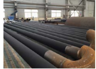
HiE-Coat™ 840-M coats gas-fired heating tubes.
