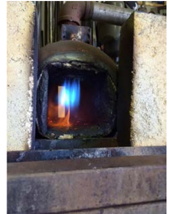
HiE-Coat™ 840-CX applied to a gas-fired forge.
