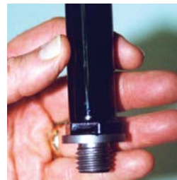
CP2000 seals thermal spray on small heater.
