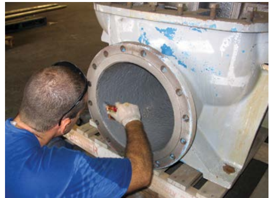
Corr-Paint™ CP2060 coats pump housing.
