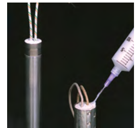
Ceramacast™ 586 pots ignitor and cartridge heater.
