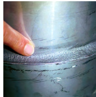
Pyro-Putty® 2400 seals high temp ducting.
