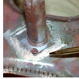
Pyro-Putty® 653 seals corroded burner manifold.
