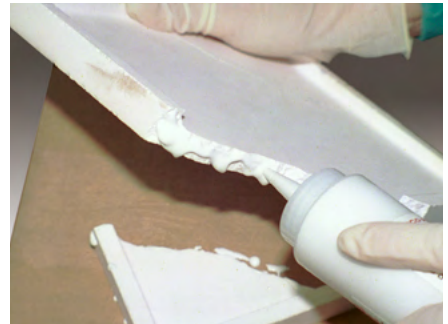
Cerabond™ 503 repairs furnace saggar plate.
