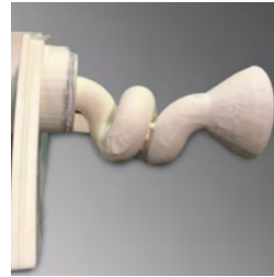
Ceramabond™ 503 coats spiral cantilevered sensor.
