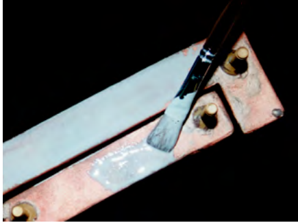
Cerabond™ 571 coats copper induction heater.
