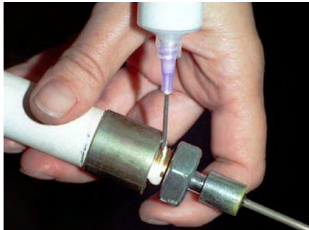
Cerabond™ 671 used as a high temp threadlocker.
