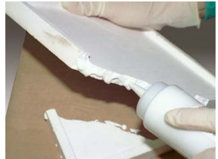
Ceramabond™ 503 repairs furnace saggar plate.
