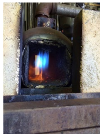
HiE-Coat™ 840-CX applied to a gas-fired forge.
