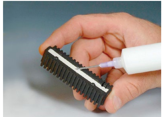
Ceramacast™ 586 pots high power resistor.
