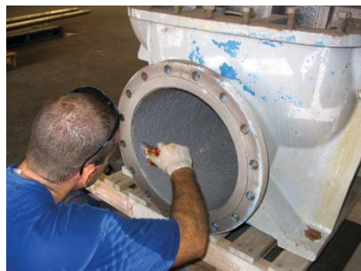
Corr-Paint™ CP2060 coats pump housing.
