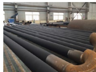
HiE-Coat™ 840-M coats gas-fired heating tubes.
