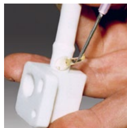
Aremco-Bond™ 526N bonds alumina to alumina ceramic.
