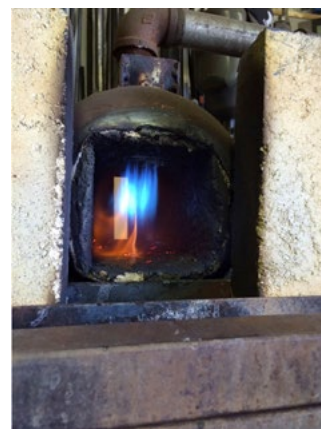
HiE-Coat™ 840-CX applied to a gas-fired forge.
