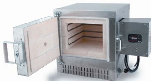
Econo-Heat™ 2928 Furnace. This model has a work area of 13" x 13 1/2" x 8 3/4" and is equipped with a single set point analog temperature controller.
