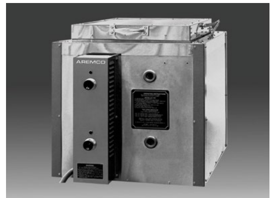
Econo-Heat™ 2931 Top-Loading Furnace. This model has a work area of 17" x 20" x 17" and is capable of 2400 °F operation using single phase service, 240 Volts and 40 Amps.
