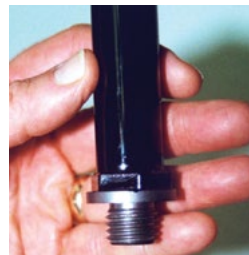
CP2000 seals thermal spray on small heater.
