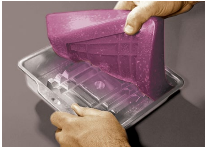
Cure the EZ-Cast™ mold and peel out your finished pliable mold.
