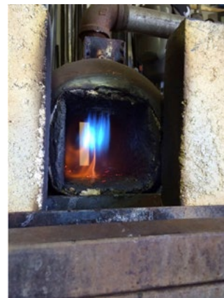
HiE-Coat™ 840-CX applied to a gas-fired forge.
