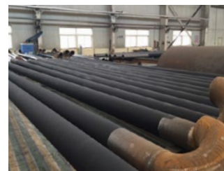
HiE-Coat™ 840-M coats gas-fired heating tubes.
