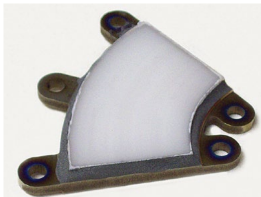
Ceramabind™ 542 seals thermal spray on sensor.
