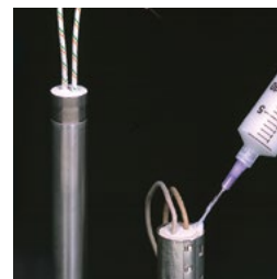
Ceramacast™ 586 pots ignitor and cartridge heater.
