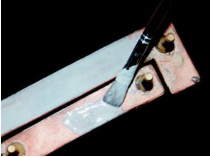
Ceramabond™ 571 coats copper induction heater.
