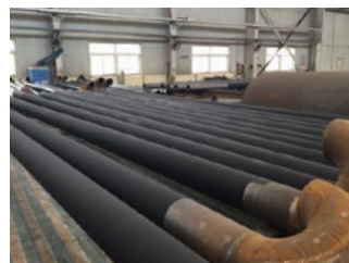
HiE-Coat™ 840-M coats gas-fired heating tubes.
