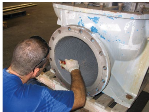
Corr-Paint™ CP2060 coats pump housing.
