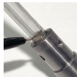
Aremco-Bond™ 631 bonds sapphire tube to stainless steel.
