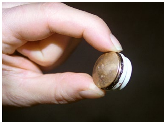
Aremco-Bond™ 570 bonds ceramic to copper nozzle.
