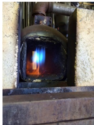
HiE-Coat™ 840-CX applied to a gas-fired forge.
