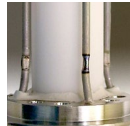
Ultra-Temp™ 516 seals heater assembly.
