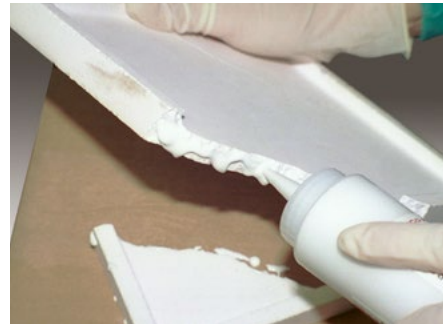
Cerabond™ 503 repairs furnace saggar plate.
