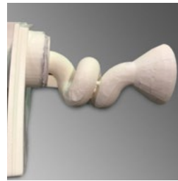
Ceramabond™ 503 coats spiral cantilevered sensor.
