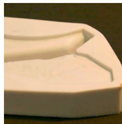
Ceramacast™ 900-N casts small, dense part.
