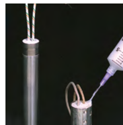
Ceramacast™ 586 pots ignitor and cartridge heater.
