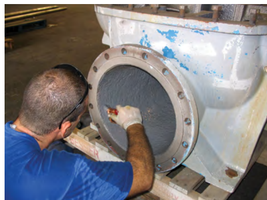
Corr-Paint™ CP2060 coats pump housing.
