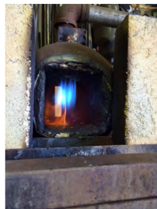
HiE-Coat™ 840-CX applied to a gas-fired forge.
