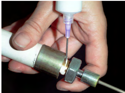
Ceramabond™ 671 used as a high temp threadlocker.
