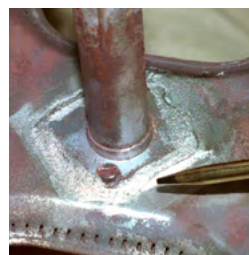
Pyro-Putty® 653 seals corroded burner manifold.
