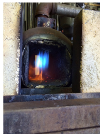
HiE-Coat™ 840-CX applied to a gas-fired forge.
