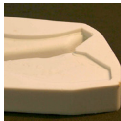
Ceramacast™ 900-N casts small, dense part.
