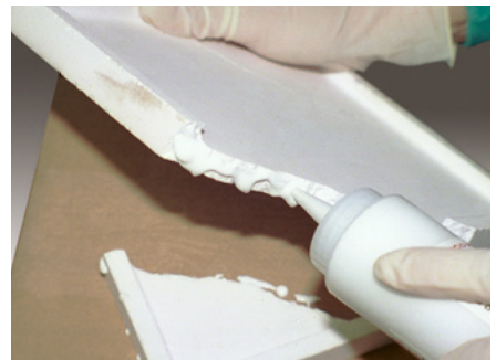
Ceramabond™ 503 repairs furnace saggar plate.
