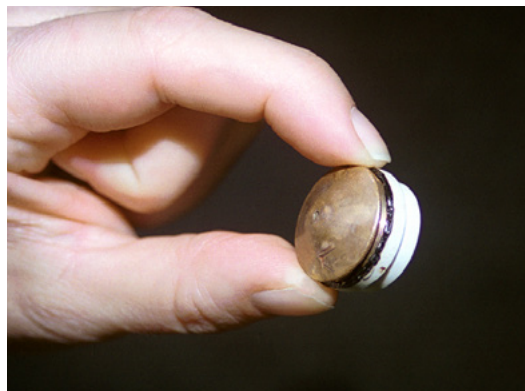
Aremco-Bond™ 570 bonds ceramic to copper nozzle.
