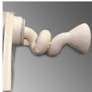
Ceramabond™ 503 coats spiral cantilevered sensor.
