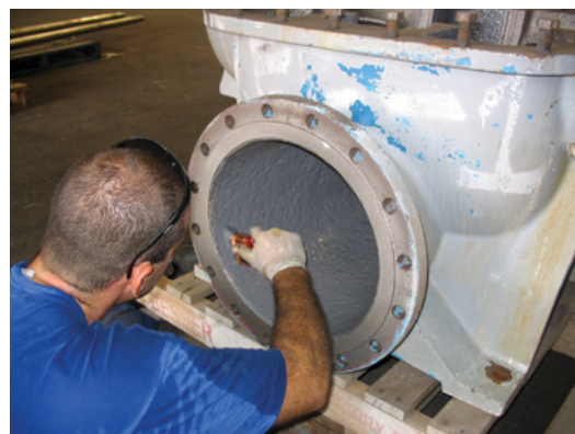
Corr-Paint™ CP2060 coats pump housing.
