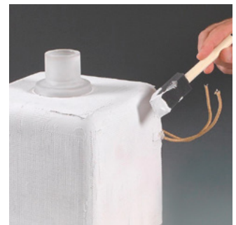
Ceramabond™ 569 bonds flex heater to quartz vessel.
