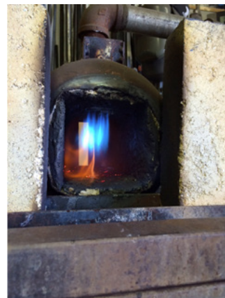
HiE-Coat™ 840-CX applied to a gas-fired forge.
