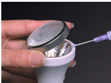
Ceramabond™ 835-M bonds cover to halogen lamp.
