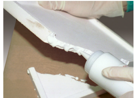
Ceramabond™ 503 repairs furnace saggar plate.
