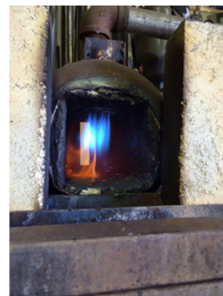
HiE-Coat™ 840-CX applied to a gas-fired forge.
