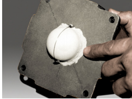
Ceramabond™ 571 coats oxygen sensor.
