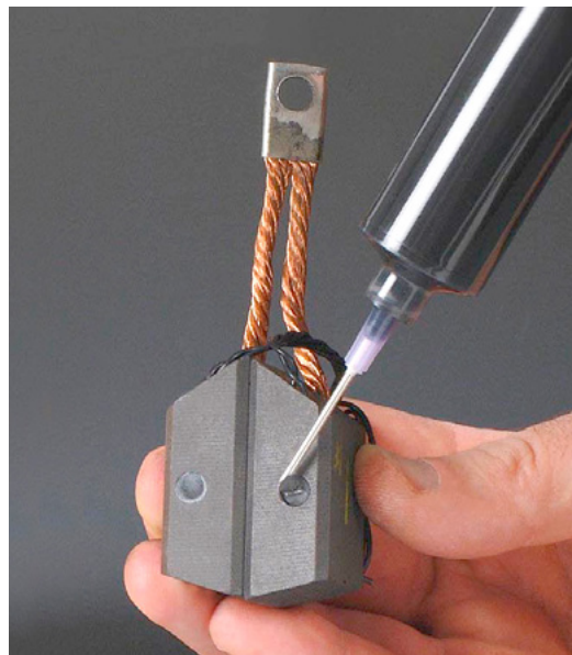
Graphi-Bond™ 551-RN seals sensor in carbon brushes.
