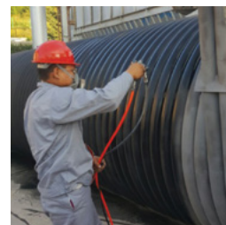
HiE-Coat™ 840-M coats industrial heat exchanger.
