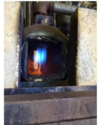
HiE-Coat™ 840-CX applied to a gas-fired forge.
