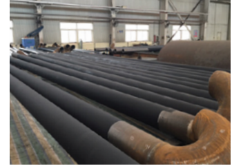
HiE-Coat™ 840-M coats gas-fired heating tubes.
