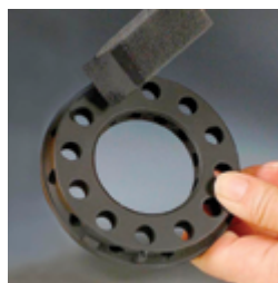
HiE-Coat™ 840-M coats gas burner component.
