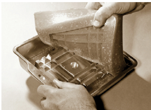
Cure the EZ-Cast™ mold and peel out your finished pliable mold.
