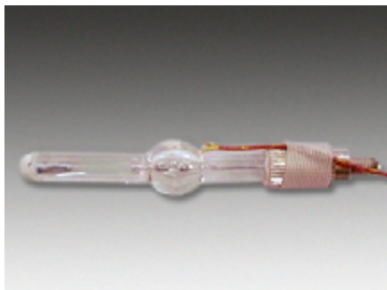
Ultra-Temp™ 516 bonds thermocouple to quartz tube.
