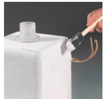
Ceramabond™ 569 bonds flex heater to quartz vessel.
