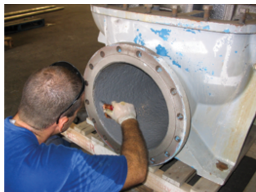
Corr-Paint™ CP2060 coats pump housing.
