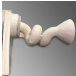
Ceramabond™ 503 coats spiral cantilevered sensor.
