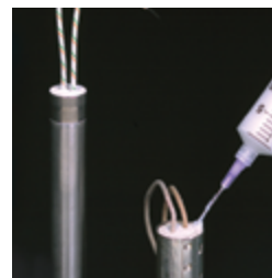
Ceramacast™ 586 pots ignitor and cartridge heater.
