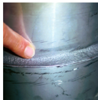
Pyro-Putty® 2400 seals high temp ducting.
