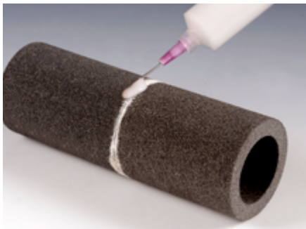
Ceramabond™ 618-N bonds porous ceramic filter elements.
