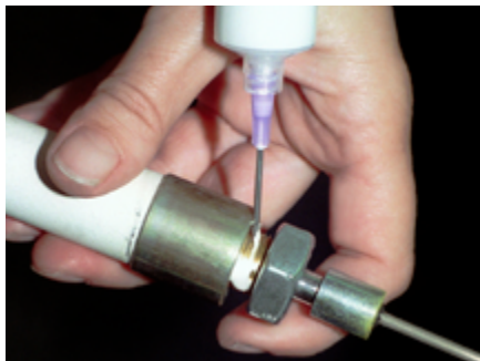
Ceramabond™ 671 used as a high temp threadlocker.
