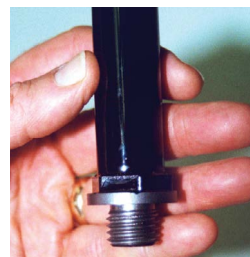
CP2000 seals thermal spray on small heater.
