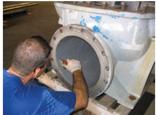
Corr-Paint™ CP2060 coats pump housing.
