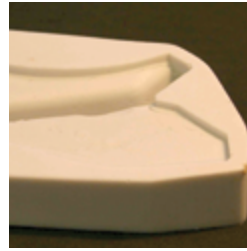
Ceramacast™ 900-N casts small, dense part.
