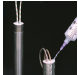
Ceramacast™ 586 pots ignitor and cartridge heater.
