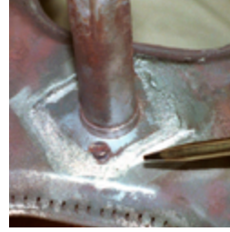
Pyro-Putty® 653 seals corroded burner manifold.
