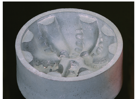
Ceramacast™ 673 mold for down-hole drill bit.
