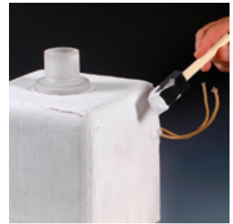
Ceramabond™ 569 bonds flex heater to quartz vessel.
