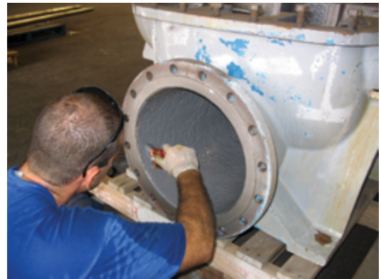
Corr-Paint™ CP2060 coats pump housing.
