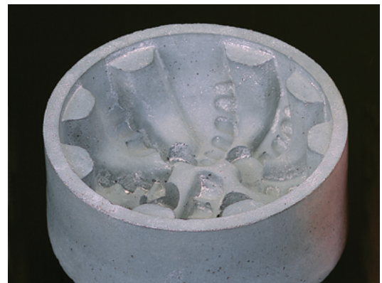
Ceramacast™ 673 mold for down-hole drill bit.
