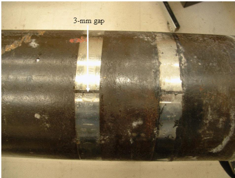
**Figure 1. Photograph of properly applied MsS strip. The corners of the strip are flush with each other and a 3 mm gap remains between the ends.**
