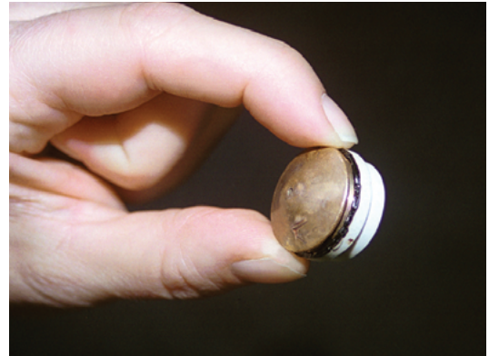
Aremco-Bond™ 570 bonds ceramic to copper nozzle.
