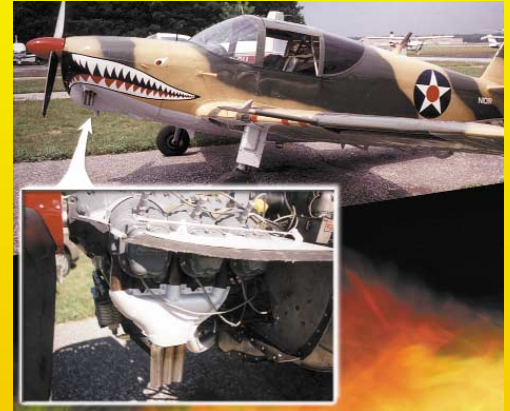
Corr-Paint™ CP3015-AL aluminum-rich, water-dispersible paint is used to coat heat shield and spark plugs on aircraft engine manifold.
