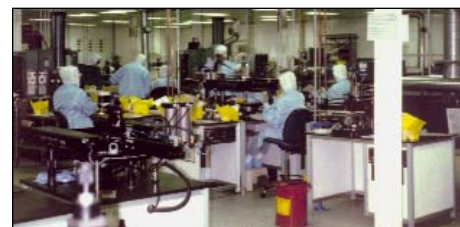
Product facility for via-filling ceramic green tape.
