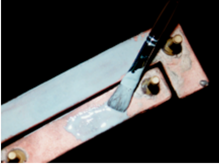
Cerabond™ 571 coats copper induction heater.
