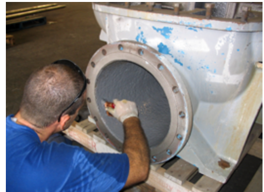
Corr-Paint™ CP2060 coats pump housing.
