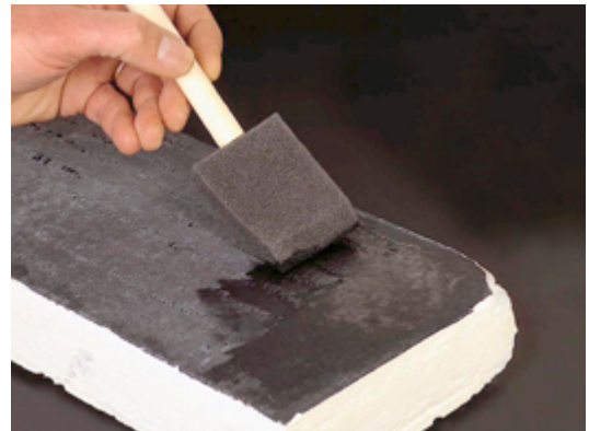
HiE-Coat™ 840-C coats ceramic fiberboard infrared heater.
