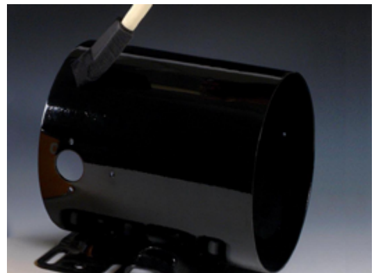
CP2000 seals thermal spray on motor housing.
