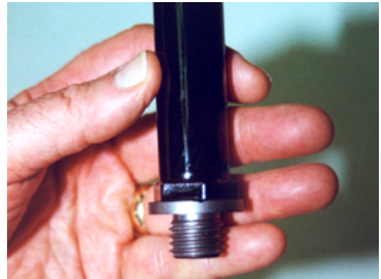
CP2000 seals thermal spray on small heater.
