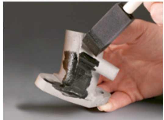
HiE-Coat™ 840-CM coats cast steel part.
