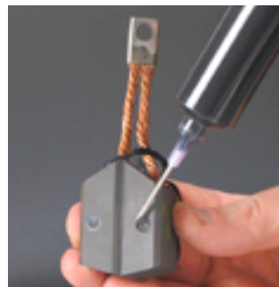
Graphi-Bond™ 551-RN seals sensor in carbon brushes.
