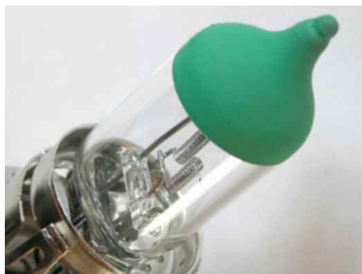
Ceramacoat™ 845-GLT applied to auto headlamp.
