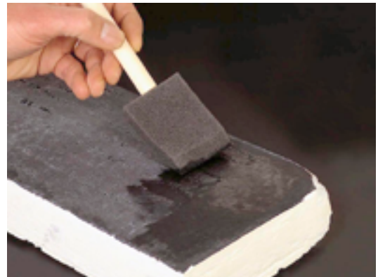
HiE-Coat™ 840-C coats ceramic fiberboard infrared heater.
