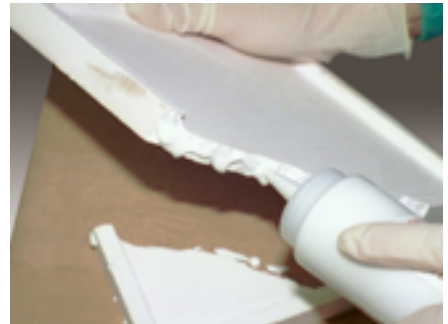
Ceramabond™ 503 repairs furnace saggar plate.
