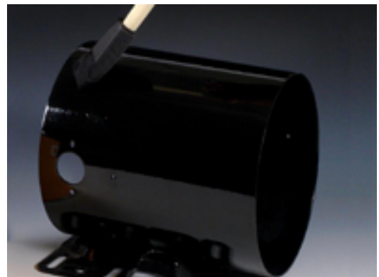
CP2000 seals thermal spray on motor housing.
