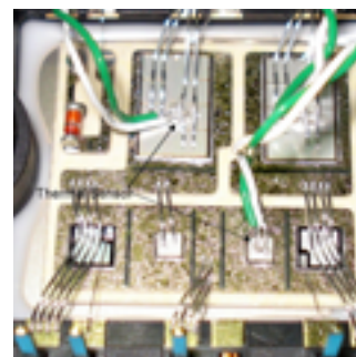
Aremco-Bond™ 556-HT-SP used to bond thermal sensor.
