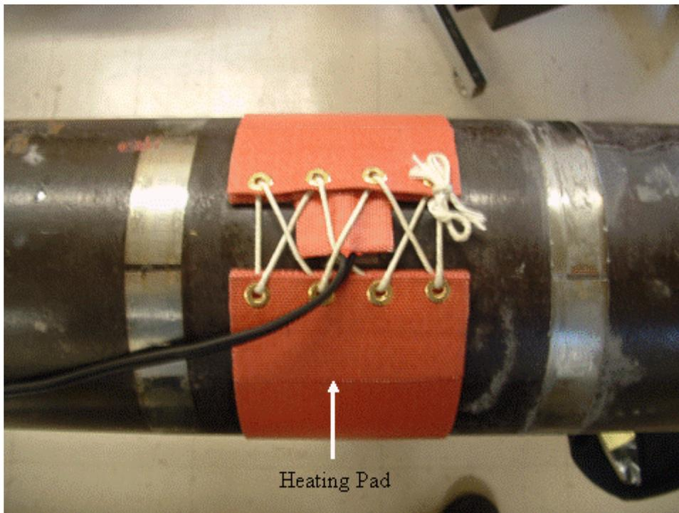
**Figure 3. Photograph of MsS strip wrapped in Watlow heating pad**
