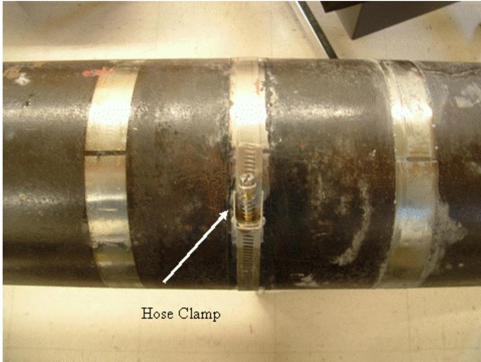
**Figure 2. Photograph of the MsS strip secured with a hose clamp for heat treatment**
