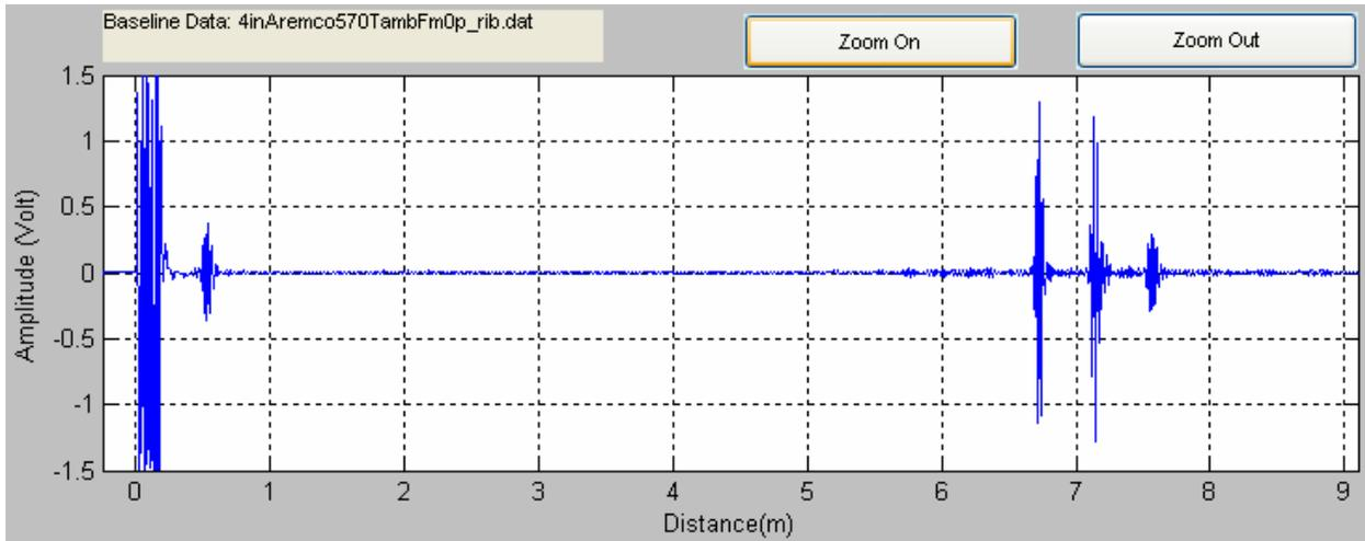
**Figure 4. Sensor quality inspection data taken on the 4-inch pipe with the sensor bonded with Aremco 570. Minimal noise is returned from the pipe and the end wall indications are narrow, showing no ringing.**
