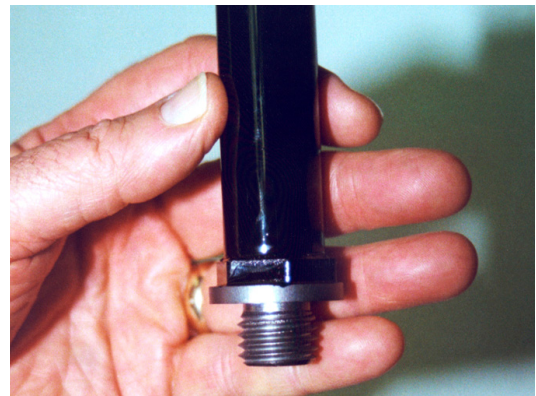
CP2000 seals thermal spray on small heater.
