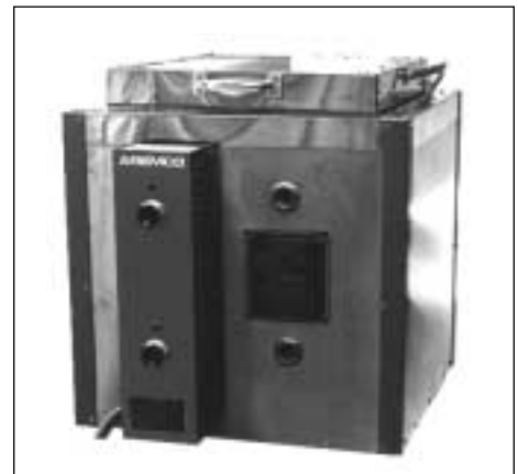
Econo-Heat™ 2931 Top-Loading Furnace. This model has a work area of 17" x 20" x 17" and is capable of 2400° F operation using single phase service, 240 Volts and 40 Amps.
