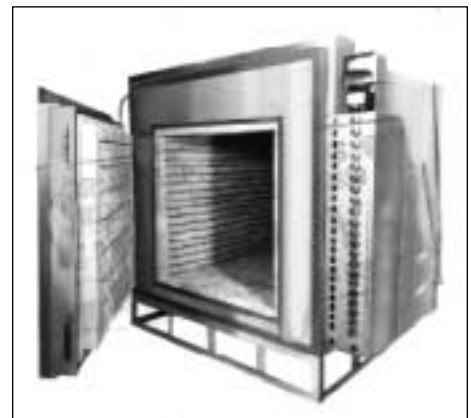
The Econo-Heat™ furnace shown is a custom unit designed for an aerospace manufacturer for use in heat treating. This furnace has a work area of 42" x 42" x 65", and a unique temperature control system consisting of 21 elements each with its own infinite control switch to permit uniform heating of complex shapes.
