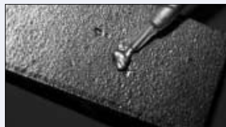
Aremco-Bond™ 657-FST repairs defects in cast iron.
