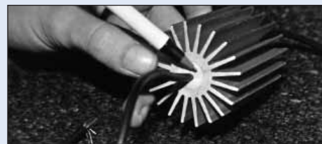
Ceramacast™ 646N seals heating apparatus.
