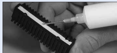
Ceramacast™ 576N pots high power resistor.
