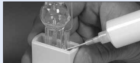
Ceramacast™ 575N pots halogen lamp.
