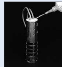
Ceramacast™ 586 used to assemble silicon carbide ignitor.
