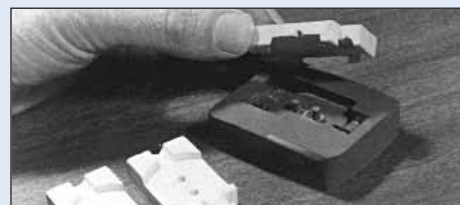
Ceramacast™ 584 casts fine detail welding fixture.
