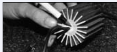
Ceramacast™ 646 seals a heat sink.
