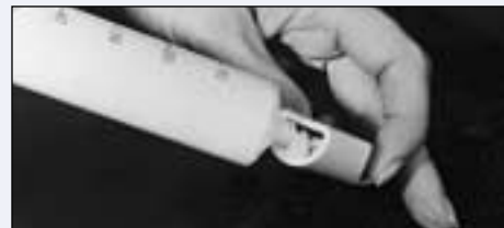
Ceramacast™ 575N insulates PTC device.
