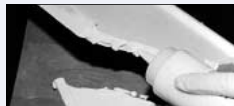
Ceramabond™ 503 repairs mullite sagger.
