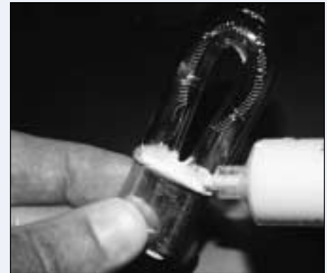
Cerabond™ 835 bonds high intensity bulb.
