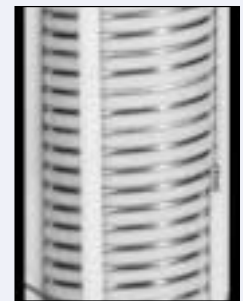
Cerabond™ 503 bonds Pt/40Rh heater wire on an alumina core. This assembly is part of a hi-temp process furnace used aboard the space shuttle.
